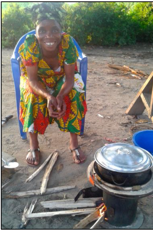
Fig. 2: A cookstove in use on the Bateke Plateau. The use of cookstoves, as opposed to the traditional three-stone open fire, could cut wood consumption in half. Photo: Lucie Escoufflaire/WCS
